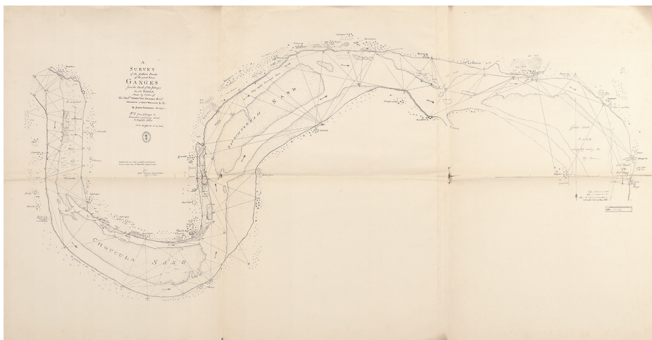
Figure 8 James Rennell, A Survey Map of the Southern Banks of the Great River Ganges , 1764–65; in this early application of trigonometric survey, Rennell, working for the East India Company, had to identify fixed objects (mostly trees) along the riverbanks to draw the imaginary line separating land and water (IOR: X/9119/3, British Library; © British Library Board).
